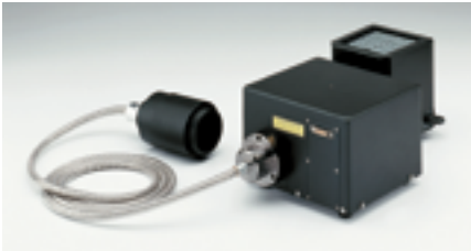
Transmitted Light Detection Unit External transmitted light photomultiplier detector and 100W Halogen conventional illumination, integrated for both laser scanning and conventional transmitted light Nomarski DIC observation. Motorized exchange between transmitted light illumination and laser detection. Simultaneous multi-channel confocal fluorescence image and transmitted DIC acquisition enabled.
