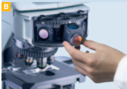
Easy replacement of filter cubes
